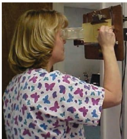
Fig. 2. A modified Brewster Stereoscope (Keystone). This version is affixed to the wall and can be adjusted to meet the needs of most people.
