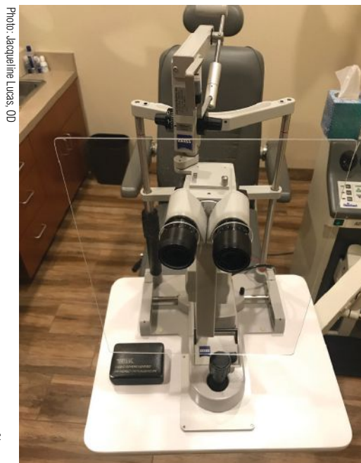
If you have the right tools, you can make your own slit lamp breath shield.
