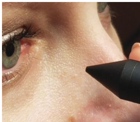
Fig. 1. A Cochet-Bonnet esthesiometer is designed for rapid assessment of corneal sensitivity.
