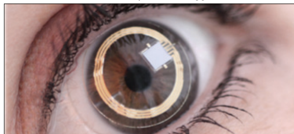
FIGURE 3. TRIGGERFISH CONTACT LENS SENSOR The Triggerfish (Sensimed) is a contact lens sensor made of a silicone contact lens that contains an embedded strain recording gauge to quantify changes in cornea curvature with IOP fluctuations.
