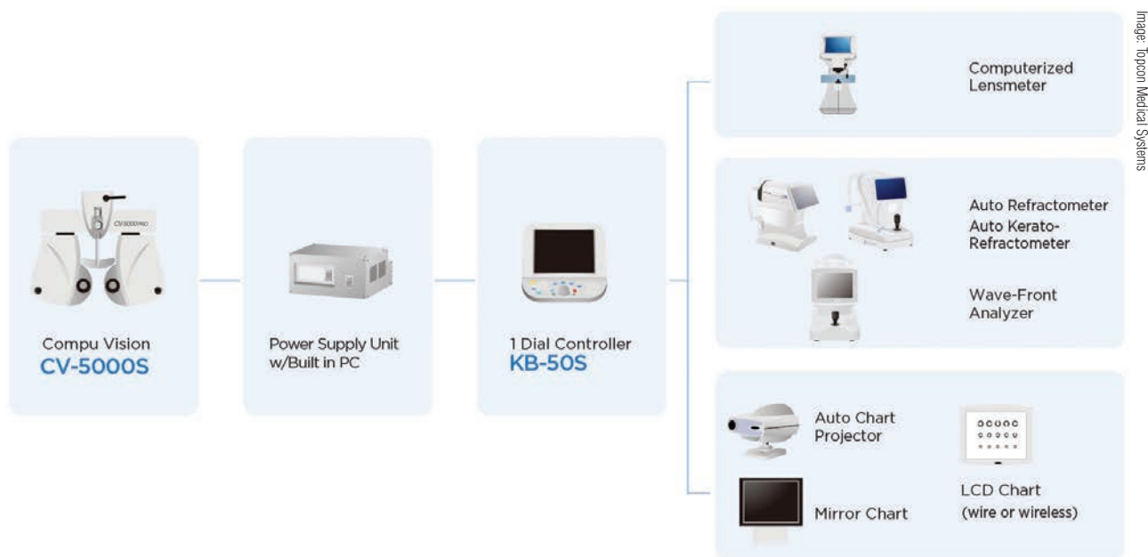
Fig. 1. This chart shows communication between various instruments in an automated refraction system.
