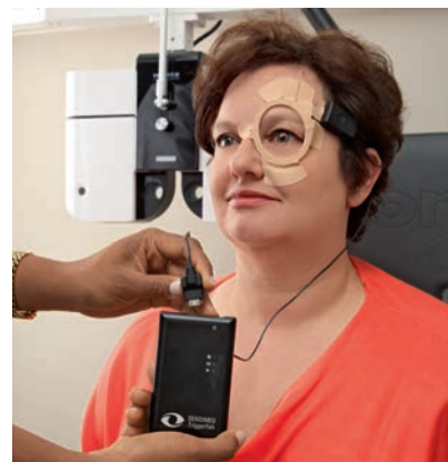
Fig. 2. Above, Sensimed’s Triggerfish for detecting ocular dimensional changes. Top right, the lens on the eye. Right, sensor data is collected by an adhesive-backed antenna worn around the eye, connected to a portable data recorder.
