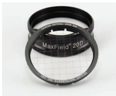
The Saxena Retinal Grid can help in estimating the size of lesions and nevi.
