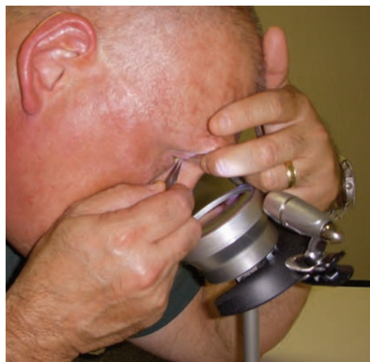
The Own Eye Magnifier was developed out of necessity. The inventor created it for his wife, who had painful trichiasis, and needed a better way to see her own eye.
