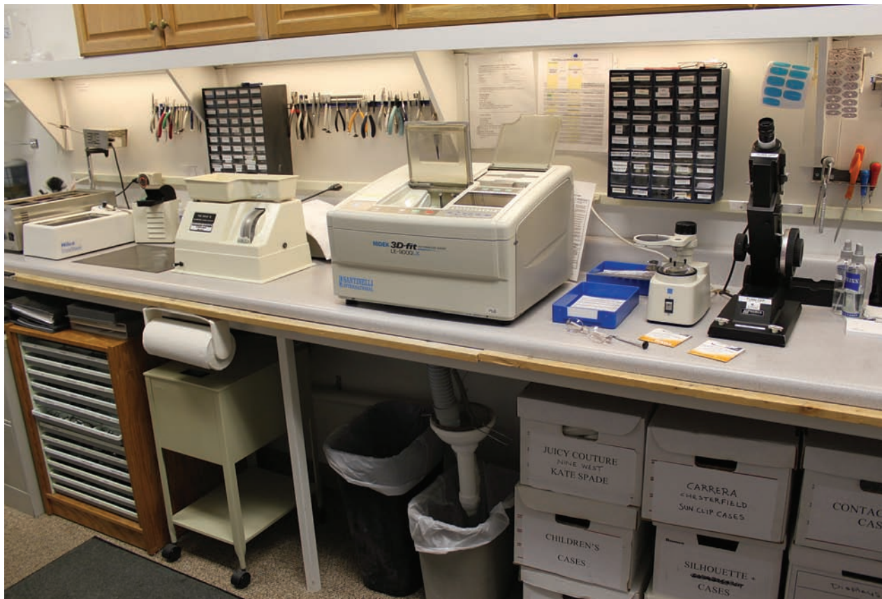
Workbench equipment is placed in order of use for convenience and efficiency. From right to left, you'll see the lensometer, a blocker, a drawer with leap blocks and roll of leap pads just above the lensometer, a work tray next to the edger, the edger, a hand-stone, the groover and the frame warmer. Notice the drain setup under the edger.
